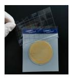
2.Place the test plate on a flat, level surface and Lift the top film.
