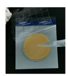
3.Dispense 1.0 mL of sample solution onto test plate center.
